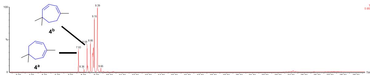
Figure S29 : GC-MS chromatogram of C 10 H 16 mixture.
