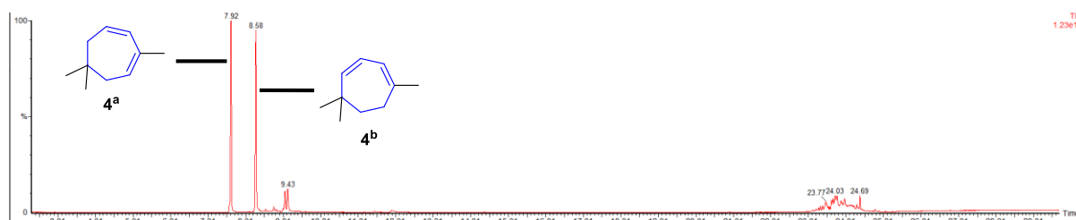
Figure S24 : GC-MS chromatogram of 4 a and 4 b mixture.
