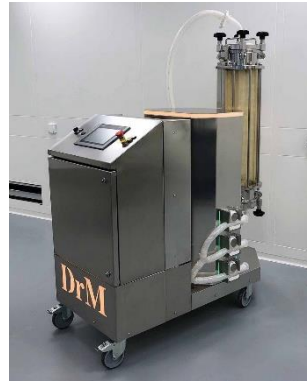
Figure 21 : Single-use alluvial filtration system from Dr. Müller AG (Pharmaceutical-technology.com, 2023).
