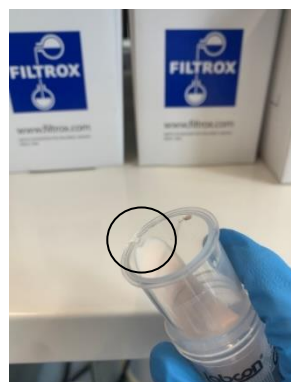
Figure 60 : Hole on the Puraspin® tube where filter aid escaped.
