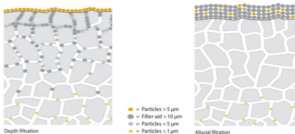
Figure 18 : Schematic description of depth and alluvial filtration (Filtrox.com 2, 2023).
