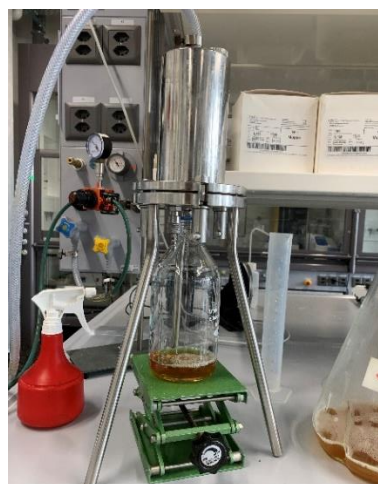
Figure 15 : Setup of a depth filtration at laboratory scale and constant pressure.
