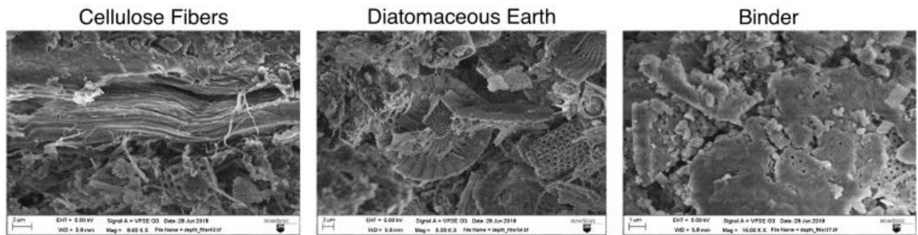
Figure 12 : The three main elements (cellulose, diatomaceous earth and a binding resin) found in depth filters under a microscope (Nejatishahidein N and Zydny AL, 2021).
