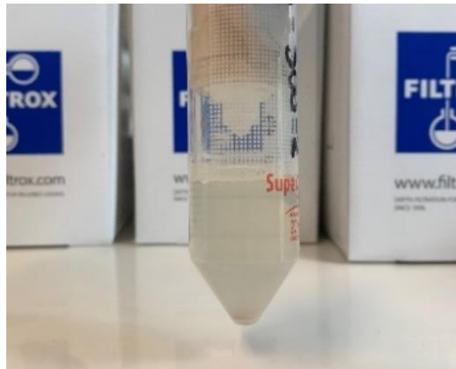
Figure 58 : A Puraspin® tube with a contaminated filtrate.
