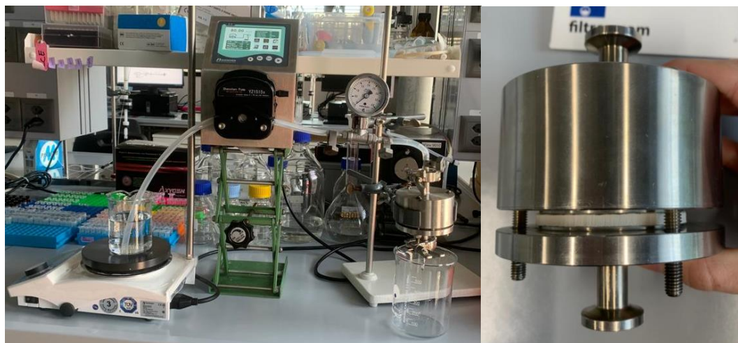
Figure 26 : Setup of the filtration with the Purafix® 2" BIO SD capsule.
