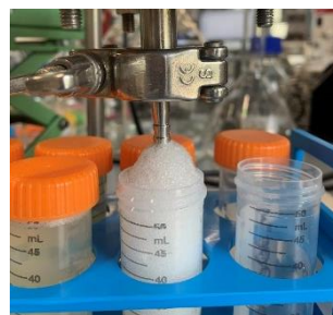
Figure 68 : Foam coming out of the capsule towards the moment the differential pressure drops quickly of Purafix® BIO SD 2" capsule filtrations.
