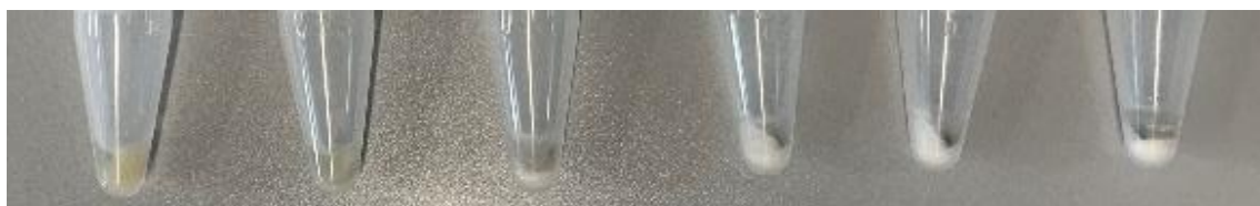
Figure 42 : Pellet of samples taken during lysis of a 4 g/L dry biomass suspension with the bead mill.
