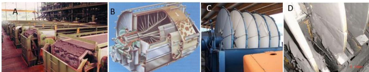
Figure 11 : Pictures of three vacuum filtration devices (A) Horizontal belt. (B) Rotating drum. (C) and (D) Rotating disc. (Crelrier S and Rüdts M, 2022).
