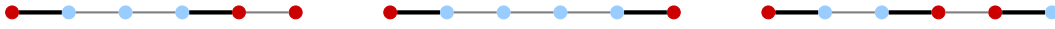
Fig. 2. The graph P_6 with a matching cut of size 2 that is not contained in a (disconnected) perfect matching (left), a disconnected perfect matching with a matching cut of size 2 (middle) and a perfect matching cut (of size 3) (right). In each figure, thick edges denote matching cut edges.
