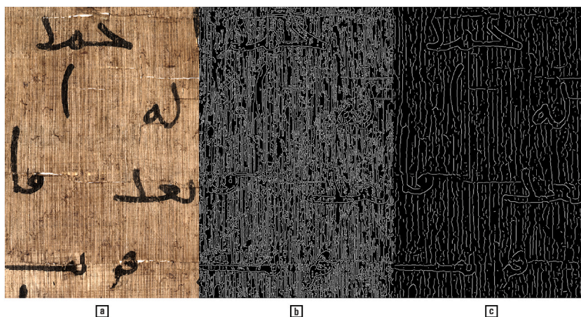
Fig. 12. (a) Colour image of a papyrus. (b) Edge detection using the Canny method for the lightness gradient [59]. (c) Applying the same method on the colour gradient. — Credits: a: Inv.Sorb. 2346, Florent Jacques, Institut de Papyrologie, Sorbonne Université, Paris.
