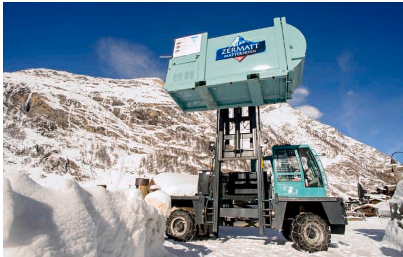
Fig. 2. Side loader vehicle carrying one container (Patent Alpenluft; SAAG).
