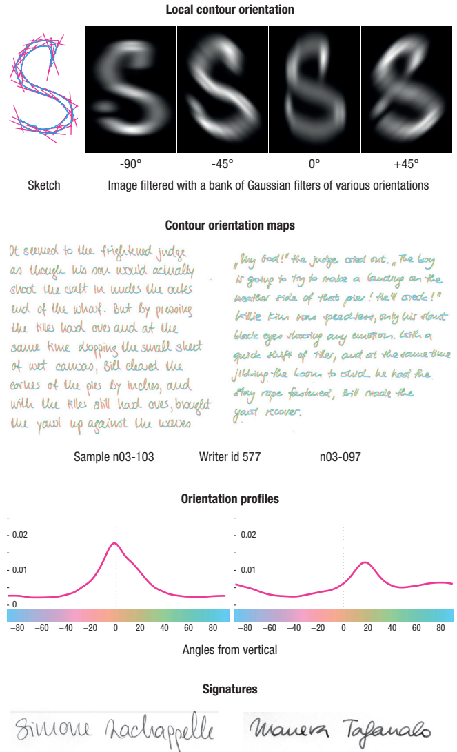
Figure 2. The orientation feature, its profile, and its analysis — A sketch illustrates the concept of local contour orientation for a single character. The anisotropic filtered images offer a peek into the process of extracting the orientation angles. Once they are obtained for each pixel along the contour, the result can be visualized by color coding the document. The orientations distribution gives the probability density function shown by a graph, where the zero angle is relative to the vertical axis of the image. — These specific handwriting samples are an example of cuckoos. The quality control system has detected a substantial difference in the measured signal, the orientation profile; visual comparison of the two samples reveals, indeed, a stylistic distinctiveness. A verification of the signatures apposed on the original forms proves the machine and human assumption: despite being labeled with the same writer id in the dataset metadata, the samples belong to different authors.
