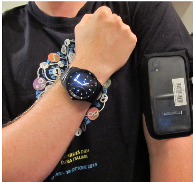
Figure 8.7. PulseCam prototype comprised of a LG G smart watch for continuously measuring one's heart rate, and a Nexus S mobile device for capturing a picture. The Nexus S is situated on one's arm using an armband.
