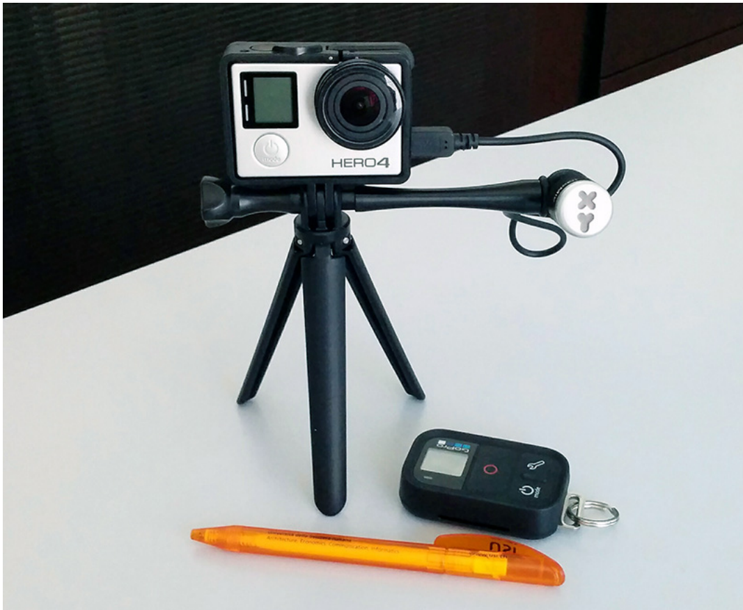
Figure 3.4. GoPro HERO4 with an external directional microphone, a tripod, and a Wi-Fi remote controller.
