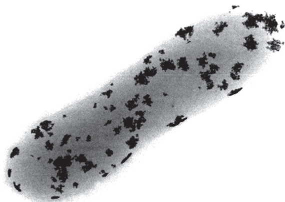
Figure 1. TEM image of platinum nanoparticles produced on the surface of the endospore of the bacteria, S. algae . Reproduced with permission. Copyright Prof. Yasuhiro Konishi, Department of Chemical Engineering, Osaka Prefecture University, Japan.
