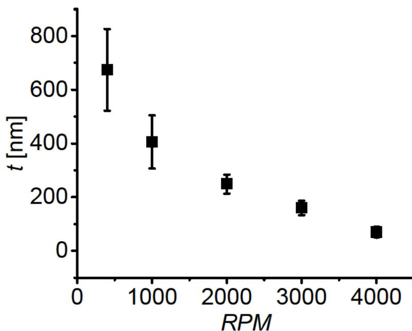
Figure S5: Film thickness  $t$  as a function of spin-coating speed for films coated from a 20% v/v monomer solution concentration.
