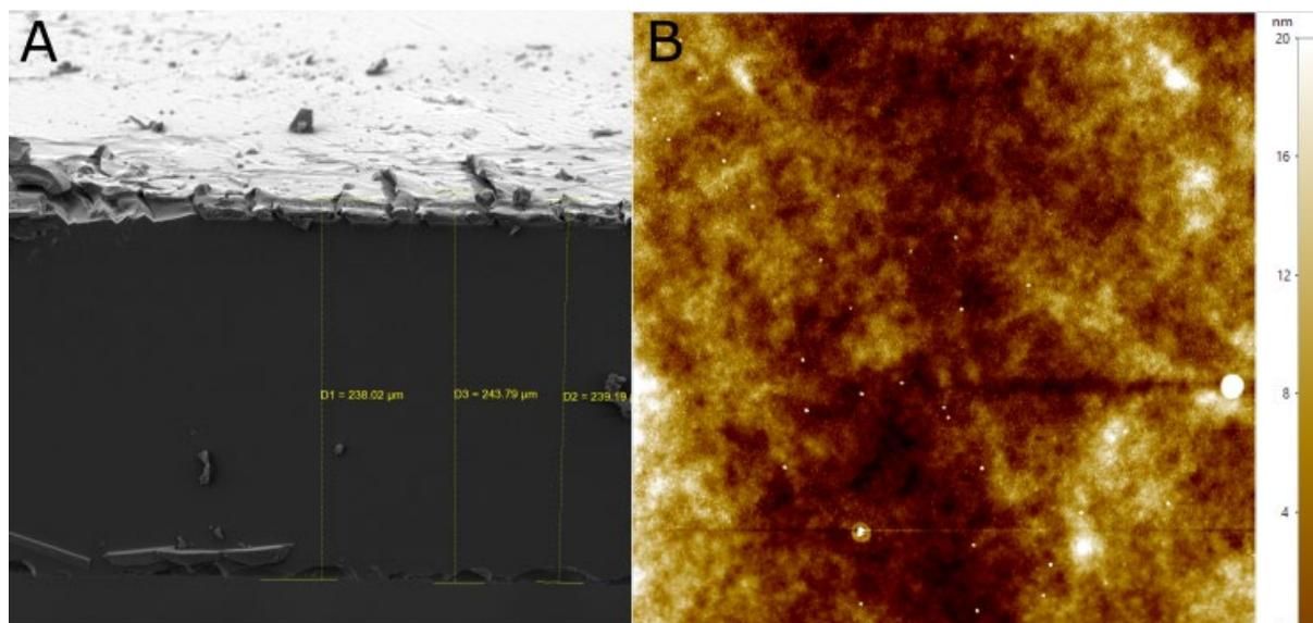
Figure S7: (A) SEM micrograph of crosssection of a thermally polymerized E3 film. (B) AFM image of the surface of a thermally polymerized E3 film.
