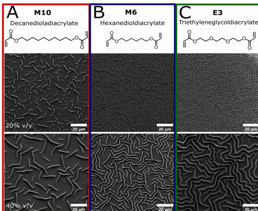
Figure S4: Chemical structures of three acrylates and the corresponding SEM images of films obtained after plasma treatment for two solution concentrations.
