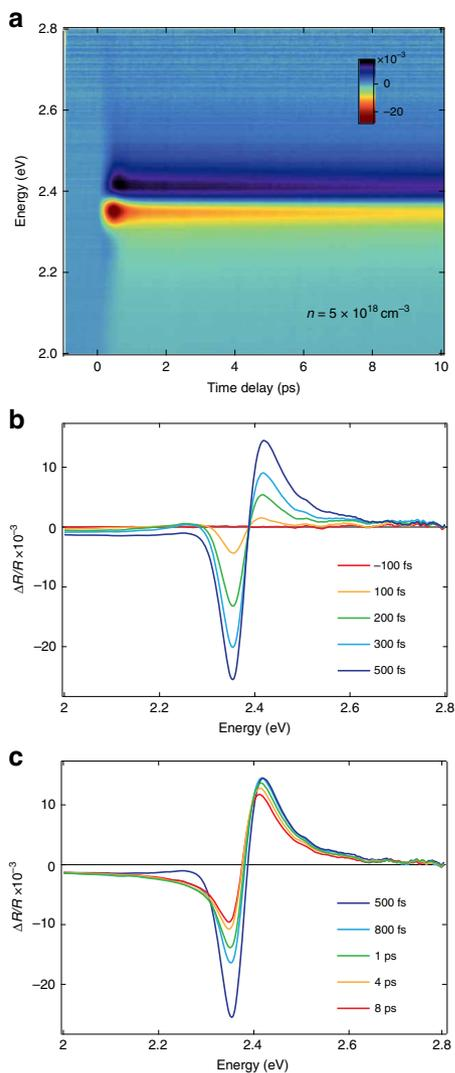
**Fig. 2 Ultrafast transient reflectivity measurements.** **a** Color-coded map of  $\Delta R/R$  as a function of probe photon energy and time delay between pump and probe. The pump photon energy is 3.10 eV and the estimated carrier density is  $n = 5 \times 10^{18} \text{ cm}^{-3}$ . The time resolution is 50 fs. **b, c**  $\Delta R/R$  transient spectra in the temporal windows **b** from  $-100$  fs to 500 fs and **c** from 500 fs to 8 ps.
