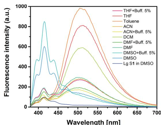
Figure 5. Solvent dependency of the fluorogenic detection of In<sup>3+</sup> (40 μM) in DCM, THF, DMF, DMSO, ACN, toluene, and their corresponding buffer (5%, Bis-Tris, 10 mM, pH 7) mixtures.
