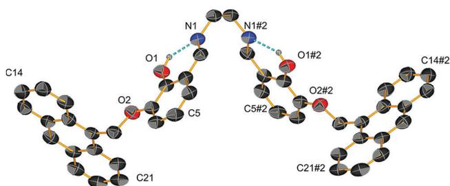
**Figure 7.** Crystal structure of sensor **S1**, ( $\#2(1/2 - x, 1/2 - y, z)$ ); H atoms are omitted except for O1–H and O1#2–H (thermal ellipsoids at 50% probability level).
