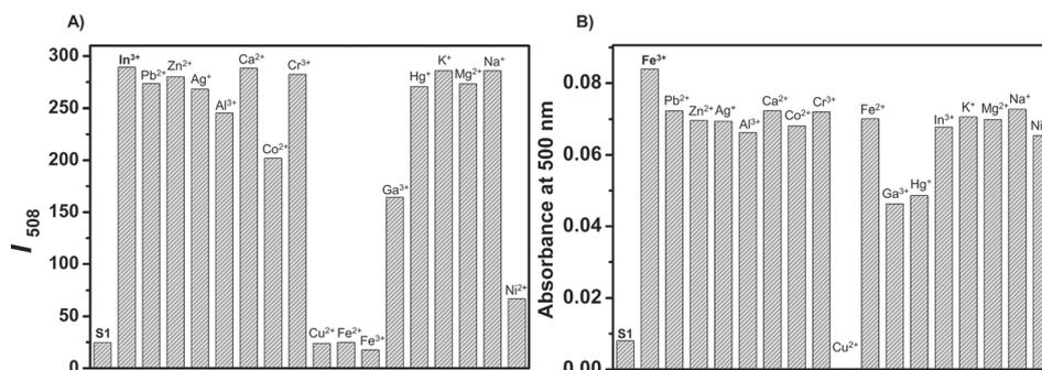
**Figure 4.** (A) Selectivity of **S1** (40  $\mu\text{M}$ ) toward  $\text{In}^{3+}$  (88  $\mu\text{M}$ , 2.2 equiv) in the presence of other metal ions (88  $\mu\text{M}$ , 2.2 equiv) in DMF ( $\lambda_{\text{ex}} = 365$  nm,  $\lambda_{\text{em}} = 508$  nm). (B) Selectivity of **S1** (40  $\mu\text{M}$ ) toward  $\text{Fe}^{3+}$  (48  $\mu\text{M}$ , 1.2 equiv) in the presence of other metal ions (48  $\mu\text{M}$ , 1.2 equiv) in DMF ( $\lambda = 500$  nm).
