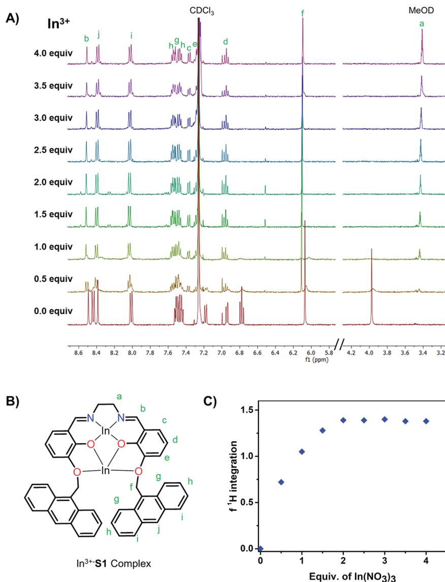
**Figure 3.** (A) Aromatic region of the <sup>1</sup>H NMR titration of **S1** with In(NO<sub>3</sub>)<sub>3</sub> (in MeOD) forming the corresponding In<sup>3+</sup>-**S1** complex at room temperature (0.5 mM) in CDCl<sub>3</sub>. (B) <sup>1</sup>H NMR proton signals assignment of the complex assignment. (C) <sup>1</sup>H NMR titration binding isotherm of the In<sup>3+</sup>-**S1** complex formation focused on the methylene-CH<sub>2</sub> bridge integrals, taking TMS as reference.
