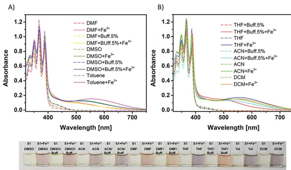
**Figure 6.** Solvent dependency of the colorimetric detection of  $\text{Fe}^{3+}$  ( $40 \mu\text{M}$ ) in (A) DMF, DMSO, and toluene and in (B) THF, ACN, DCM, and their correspondent buffer (5%, Bis-Tris, 10 mM, pH 7) mixtures.
