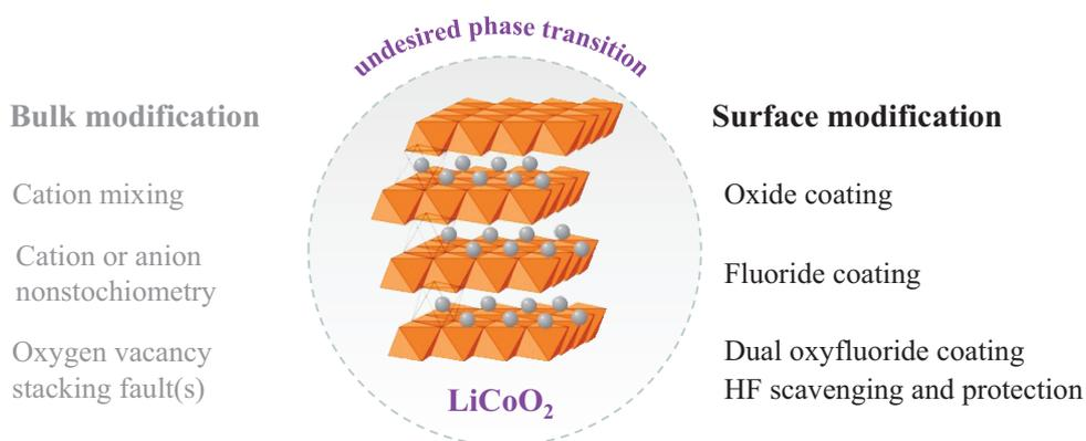
– representative of layered transition metal oxide positive-electrode materials
