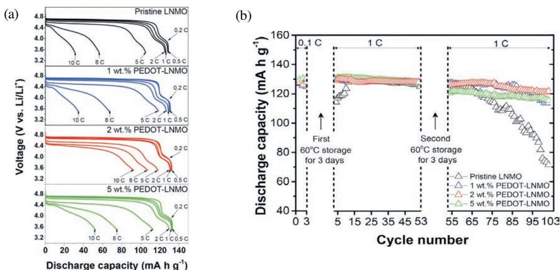
Fig. 12. (a) Rate capability and (b) cycle performances combined with the storage test of the pristine LNMO and PEDOT coated LNMO. The storage test at 60 °C for 3 days was performed after the charging process up to 4.9 V. ref. [86] Copyright 2018, American Chemical Society.
