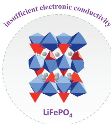
– representative of olivine-type positive-electrode materials  $\text{LiMPO}_4$  ( $M = \text{Co}, \text{Fe}, \text{Mn}, \text{Ni}$ )
