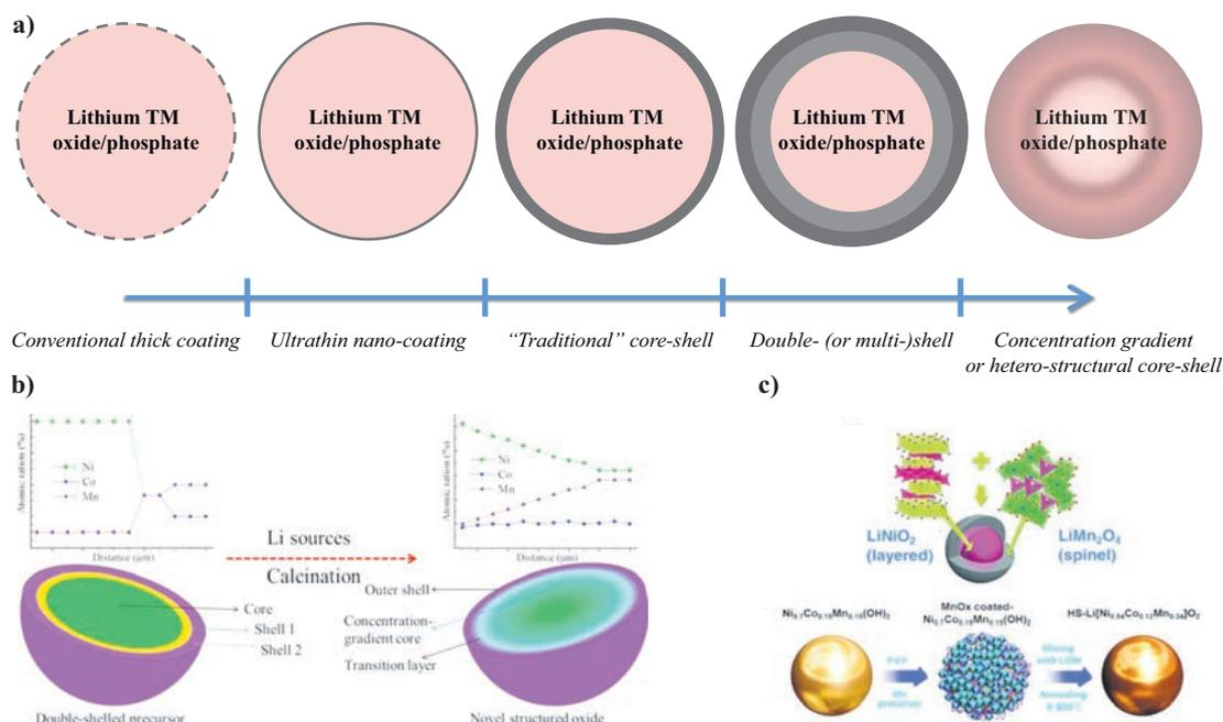
Fig. 2. (a) Schematic illustration of different coating methods applied to positive-electrode materials, a concept adapted from ref. [17]. (b, c) Preparation of double and concentration-gradient-shelled positive-electrode materials, reprinted with permission from ref. [18]. Copyright 2015 American Chemical Society. (c) Formation of heterostructured core-shell particles, reproduced from ref. [19a] with permission from John Wiley and Sons.
