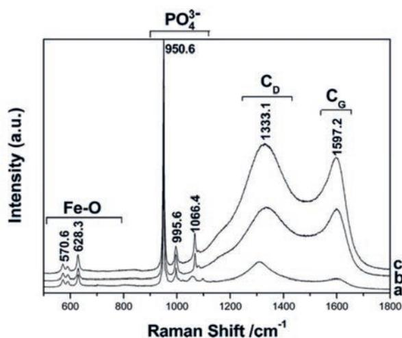
Fig. 6. Raman spectra of the as-sintered  $\text{LiFePO}_4\text{-C}$  with different carbon content: 0.5 wt% (a), 2.0 wt% (b), and 3.0 wt% (c) of Poly(vinyl alcohol). Reprinted with permission from ref. [46]. Copyright (2008) American Chemical Society
