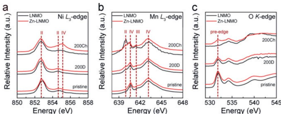
Fig. 7. sXAS TEY (total electron yield) spectra of different LMNO and Zn-LMNO electrodes tested before cycling and after 200 cycles at both charged (200Ch) and discharged (200D) states. (a) Ni L<sub>3</sub>-edge sXAS spectra. (b) Mn L<sub>3</sub>-edge sXAS spectra. (c) O K-edge sXAS spectra. Reprinted with permission from ref. [50]. Copyright (2019) American Chemical Society
