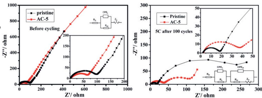
Fig. 9. Nyquist plots of pristine  $\text{Li}[\text{Li}_{0.2}\text{Fe}_{0.1}\text{Ni}_{0.15}\text{Mn}_{0.55}]\text{O}_2$  sample and  $\text{AlPO}_4$ -coated one before and after 100 cycles at 5C (AC-5:  $\text{AlPO}_4$  coating of 5 wt%). Reprinted with permission from ref. [43a]. Copyright (2015) American Chemical Society
