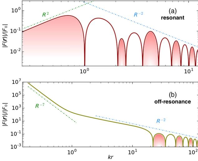
FIG. 1. *Forces between nonabsorbing particles.* Log-log plot of the absolute value of the interaction force between nonabsorbing particles with  $\alpha$  given by Eq. (3), with  $\omega_0 = 0.1\omega_F$ ,  $\Gamma_0 = 0$ , and  $a = \lambda_F/100$  for (a) the resonant frequency  $\omega = \omega_F$  and (b) strongly off resonance  $\omega = 0.1\omega_F$ . Red shadowed regions indicate repulsive interaction force.
