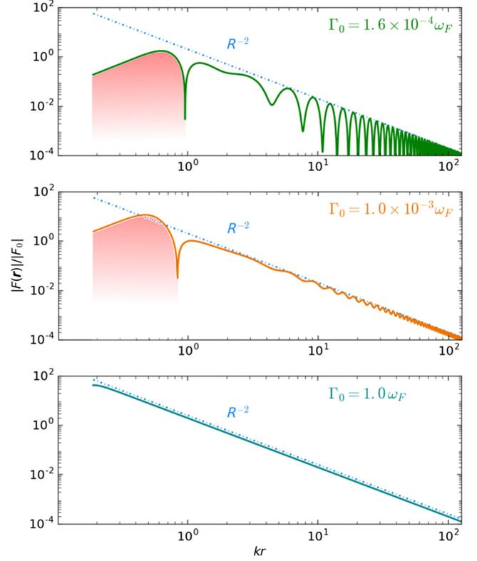
FIG. 2. *Forces between absorbing particles.* Log-log plot of the absolute value of the interaction force between absorbing particles with  $\alpha$  given by Eq. (3), with  $\omega_0 = 0.1\omega_F$ ,  $\omega = \omega_F$ , and  $a = \lambda_F/100$  for different damping coefficients (shown in each plot). Red shadowed regions indicate repulsive interaction force.
