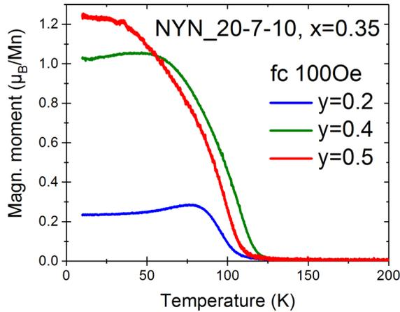
FIG. 5. Magnetization vs temperature curves of the series of NCSMO(20 nm)/YBCO(7 nm)/NCSMO(10 nm) trilayers with  $x = 0.35$  with different Sr-content,  $y$ , obtained during field-cooling (fc) in 100 Oe applied parallel to the film plane. It shows that the ferromagnetic moment grows continuously as  $y$  increases and the Mn-CO/OO becomes weaker.
