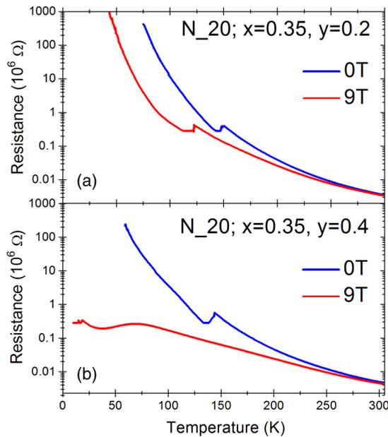
FIG. 3. Magnetoresistance vs temperature curves of  $\text{Nd}_{1-x}(\text{Ca}_{1-y}\text{Sr}_y)_x\text{MnO}_3$  single layers with  $x = 0.35$  and (a)  $y = 0.2$  and (b)  $y = 0.4$ .
