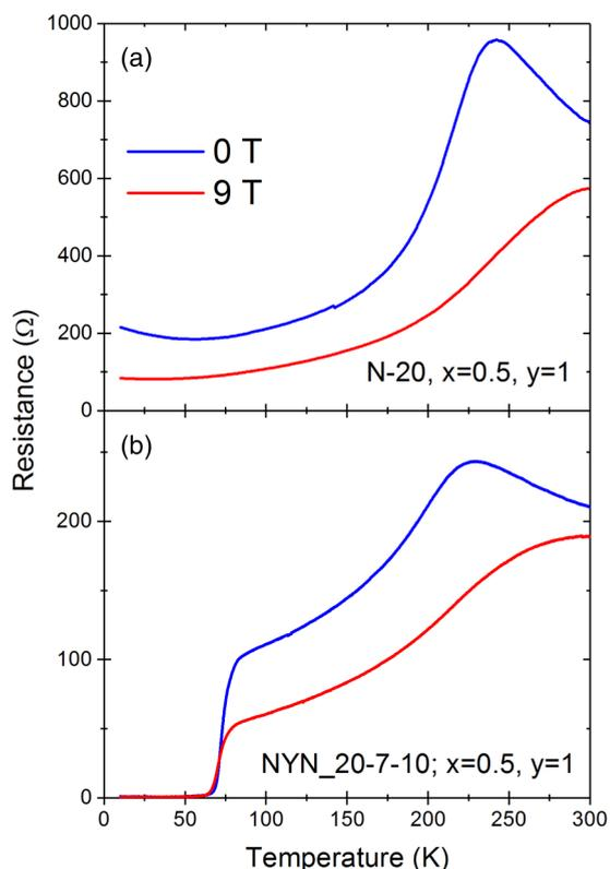
FIG. 8. Magnetoresistance vs temperature curves of (a) a NCSMO(20 nm) single layer with  $x = 0.5$  and  $y = 1$ , and (b) a corresponding NCSMO(20 nm)/YBCO(7 nm)/NCSMO(10 nm) trilayer with  $x = 0.5$  and  $y = 1$ . The trilayer exhibits a regular superconducting transition already in zero magnetic field, and the major magnetic field effect occurs in the normal state due to the magnetoresistance of the NCSMO layer.
