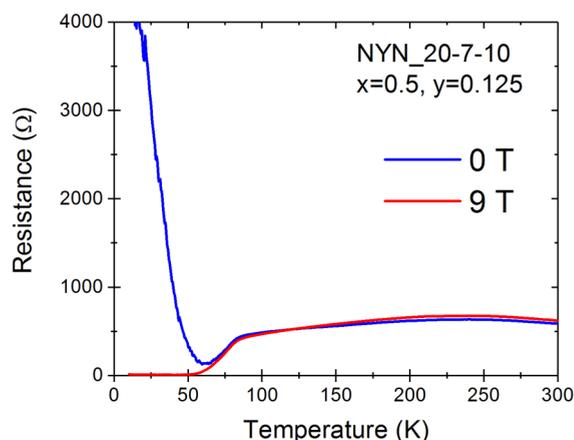
FIG. 7.  $R$ - $T$  curves of the NCSMO(20 nm)/YBCO(7 nm)/NCSMO(10 nm) trilayer with  $x = 0.5$  and  $y = 0.125$ , which exhibits a magnetic-field-induced transition from a low-field state with an insulator-like low-temperature response to a high-field state with a regular superconducting transition.
