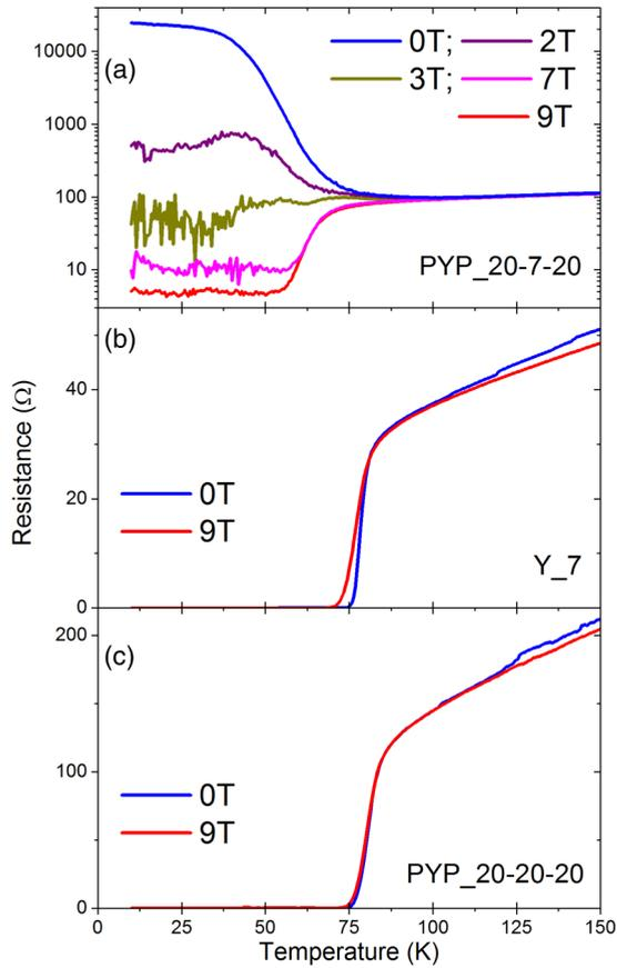
FIG. 1. Magnetoresistance vs temperature curves of thin films and multilayers from  $\text{Pr}_{0.5}\text{La}_{0.2}\text{Ca}_{0.3}\text{MnO}_3$  (PLCMO) and  $\text{YBa}_2\text{Cu}_3\text{O}_7$  (YBCO). (a) For a PLCMO(20 nm)/YBCO(7 nm)/PLCMO(20 nm) trilayer that was already discussed in Ref. [36], (b) for a YBCO(7 nm) single layer, and (c) for a PLCMO(20 nm)/YBCO(20 nm)/PLCMO(20 nm) trilayer.
