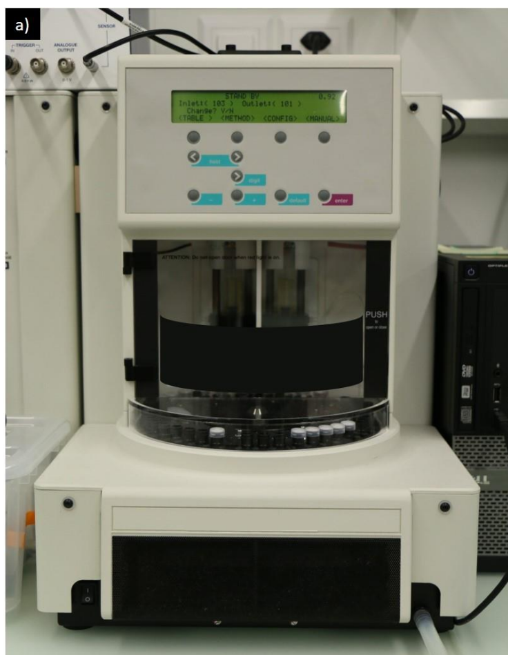
Scheme S1. Top: The layout of our TDA instrument, where the basic operation is alike to that of liquid chromatography. A pressure-driven laminar flow carries the injected sample taken from a temperature-controlled sample tray, and the optical extinction of the dispersed band is observed at fixed position along the capillary, using a selected wavelength by means of a set of exchangeable filters. In many cases, one obtains two detection points by looping the capillary. Bottom: a) The main housing and front panel of the instrument. b) The illumination and detection unit inserted from top. c) The illumination and detection unit securing the capillary loop.
