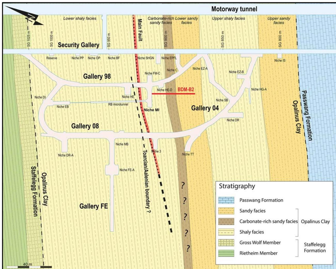
**Fig. 3** Map of the Mont Terri rock laboratory with distribution and thicknesses of major lithofacies. Position of the BDM-B2 core is indicated in red. A major fault (Main Fault) is indicated within the
