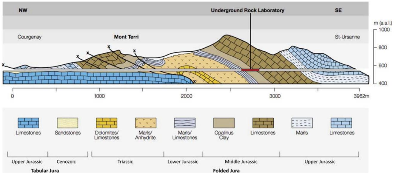
Fig. 2 Simplified geological profile along the Mont Terri motorway tunnel. The location of the Mont Terri rock laboratory is indicated in red. Positions of the main faults are indicated. Modified after Freivogel and Huggenberger (2003)
