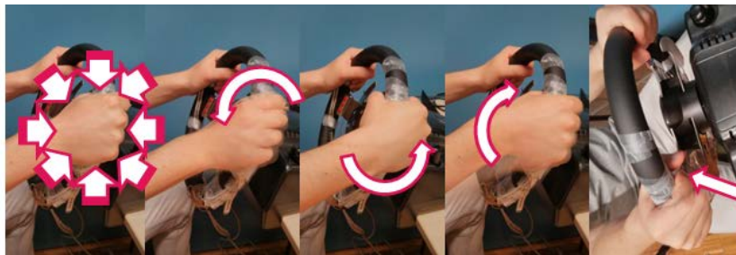
Figure 34. The five gestures for the hybrid WheelSense system. From left to right, hand squeeze, dragging downward, dragging upward, hand press, index tap.
