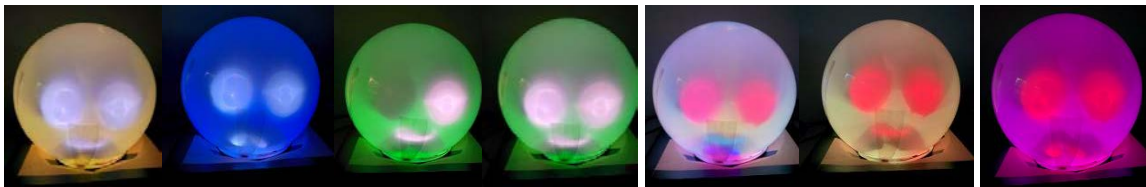
Figure 49. The five emotional states of the ADA lamp: happy, sad, trusty (eye blink) (2x), ecstasy (2x) and angry.
