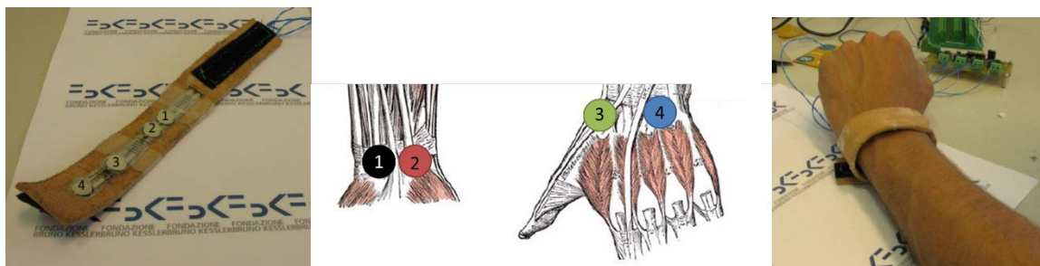
Figure 60. On the left, the wrist strap with four FlexiForce sensors mounted on it; in the center, the placement of the sensors in relation to sensors; on the right, the strap wore on the wrist and the conditioning electronics.
