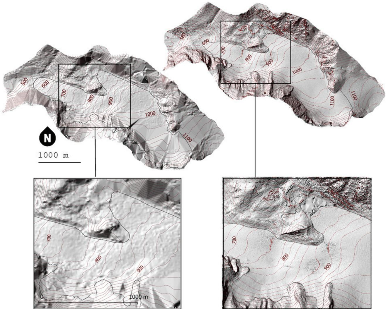
**FIGURE 4.** 1985 (left) and 2014 (right) DEMs with 25 m contour lines as well as the respective glacier outlines. Magnified sections of the DEMs are shown to highlight the difference in resolution and accuracy between the two models.
