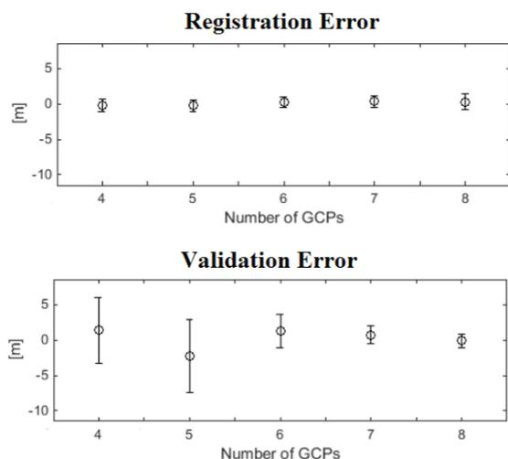
**FIGURE 5.** Registration and validation errors as functions of the number of the GCPs. Error bars represent residuals' variance. Note that the glacier surface area covered by the GCPs is proportional to their number. While the registration error does not depend on the number of GCPs, the validation error and its standard deviation decrease with an increasing number of GCPs. At eight GCPs the validation and registration errors become very similar.
