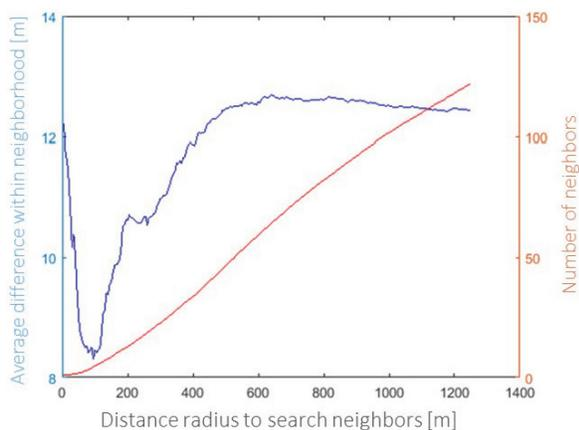
**FIGURE 6.** Average deviation of surface lowering (1985 to 2014) at the manually selected points, expressed as a function of horizontal distance. For a neighborhood distance of 100 m, the deviation is minimal, that is, 8.4 m. On average, we find 4.5 neighboring points within 100 m.
