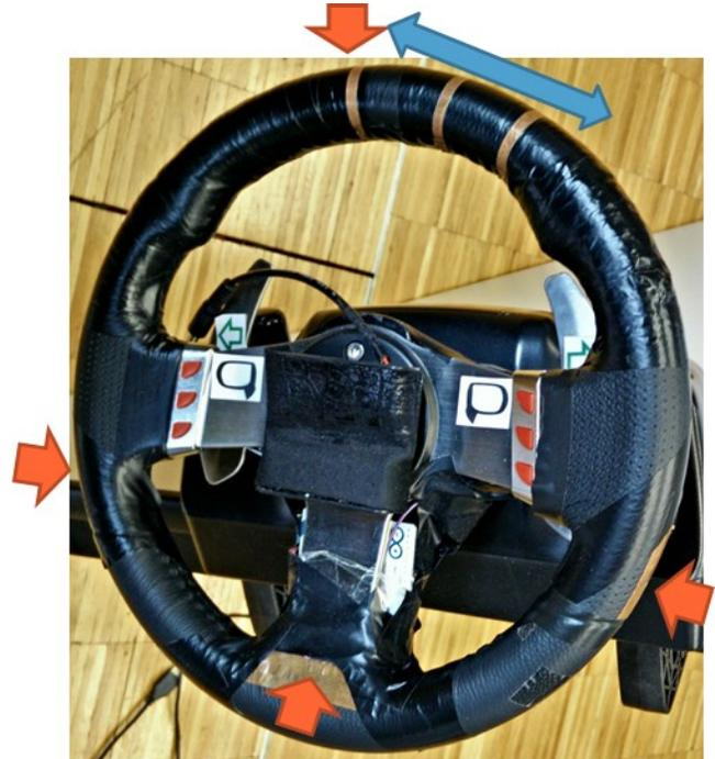
**Figure 2. Logitech G27 Steering Wheel equipped with capacitive sensors, also called WheelSense. Red arrows depict hand-taps and blue arrow the hand-swipe.**
