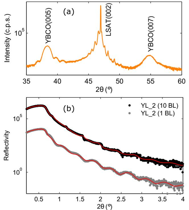
FIG. 1. (a) Symmetric  $\theta$ - $2\theta$  x-ray diffraction curve of YL\_2 (with 10 BL repetitions) along the [00L] direction. Thickness oscillations around the high intensity Bragg peaks testify for the quality of the ML. (b) X-ray reflectivity profiles (symbols) for YL\_2 type samples with 1 and 10 BL repetitions. The solid red lines are the best fits to the data.
