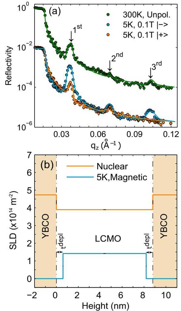
FIG. 6. (a) Polarized neutron reflectometry data (symbols) for YL<sub>2</sub> in the nonmagnetic state at 300 K and the FM state at 5 K. Also shown are the best fits (solid lines) using a blocklike depth profile of the nuclear and magnetic potentials. (b) The deduced nuclear (orange) and magnetic (blue) depth profiles in units of the scattering length density (SLD). The magnetic moment in the central part of LCMO amounts to about  $3 \mu_B$  per Mn ion.
