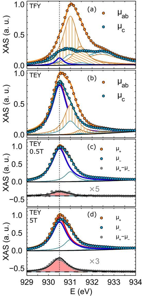
FIG. 12. Cu XAS curves of YL3 with the linear polarization of the x rays parallel and perpendicular to the CuO<sub>2</sub> planes in the (a) TFY and (b) TEY modes. Cu XAS curves of YL3 for circular polarizations and the corresponding XMCD signals at (c) 0.5 T and (d) 5 T.
