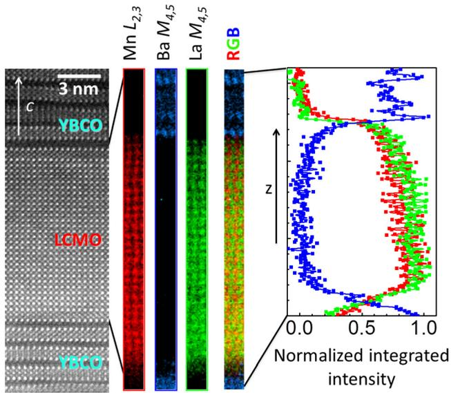
FIG. 2. Left panel: Atomic resolution, Z-contrast high-angle annular dark field image of the YBCO/LCMO/YBCO stacking in a YL\_2 type sample. Right panel: Elemental maps obtained from the analysis of the Mn  $L_{2,3}$  (red), Ba  $M_{4,5}$  (blue), and La  $M_{4,5}$  (green absorption edges). An RGB overlay of the three maps, along with a line profile on a matching color scale of the normalized integrated intensities, is also shown. Some spatial drift is visible.
