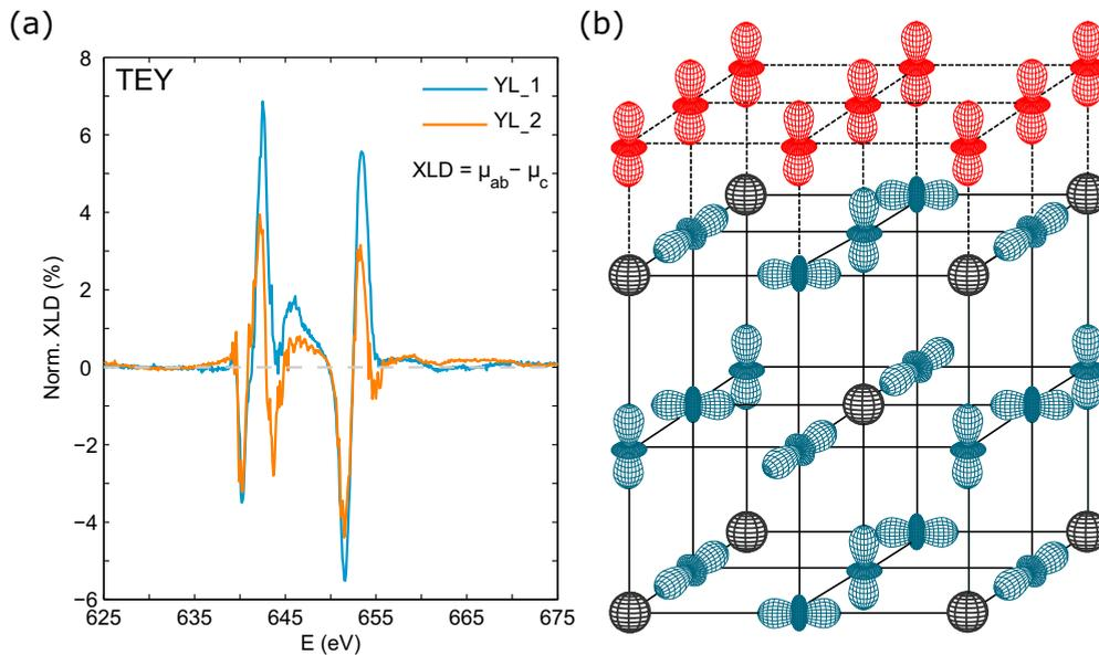
FIG. 9. (a) Mn XLD curves in TEY mode of YL\_1 and YL\_2 showing the larger orbital polarization in the former. (b) Sketch of the LCMO/YBCO interface for a lattice of the orbital polarons (in a FM state at 25% hole doping). For YBCO only the  $3d_{3z^2-r^2}$  orbitals (red) are shown which participate in the exchange interaction.
