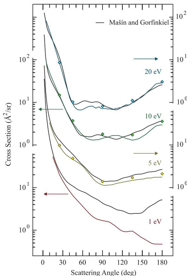
FIG. 4. Comparison of the present experimental DCS (colored lines) with the calculated results of Mařín and Gorfinkiel (Ref. 3 and this work) (black lines). Diamonds indicate sums of elastic and vibrationally inelastic (all modes) cross sections.
