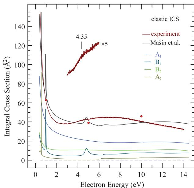
FIG. 8. Comparison of the experimental ICS with the calculated results (without Born correction) of Mašín *et al.* (Ref. 3 and this work). The contributions of all symmetries are indicated.
