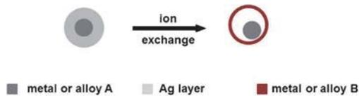
Figure 8. Preparation of nanorattles by galvanic replacement.
