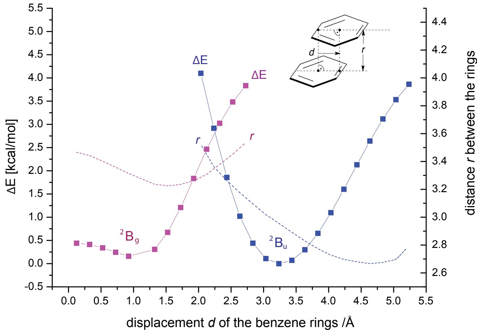
The benzene dimer cation: potential surfaces for x-displacement (from UB3LYP/6-31G\* calculations)
