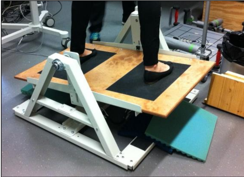
Abb. 11: Stabilometer (stability platform, Model 16030, Lafayette, IN, USA).
