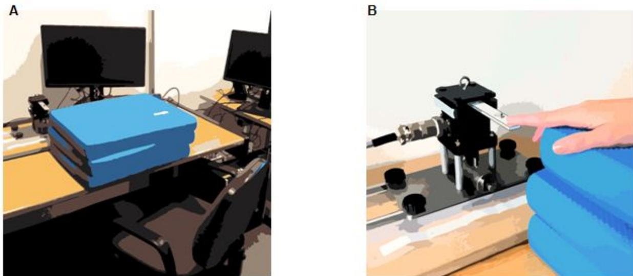
**Fig. 15: The visuomotor accuracy-tracking task (AT).** A. Setup for the AT. B. Arm and hand support structure with finger place on the lever.
