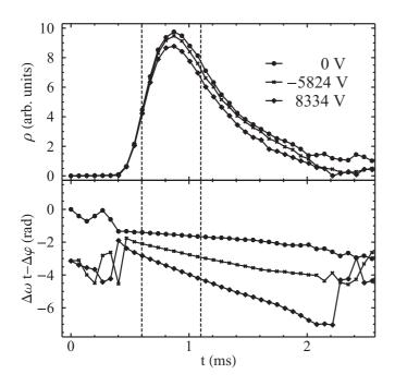
FIG. 9. Time-of-flight distribution  $\rho(t)$  (top) and phase  $\Delta \omega t - \Delta \varphi$  (bottom), obtained by Fourier transformation of the Ramsey signals under different electric-field conditions. Data between the vertical dashed lines were used to infer the frequency  $\Delta \omega(U)$  and phase  $\Delta \varphi(U)$  shifts of interest.
