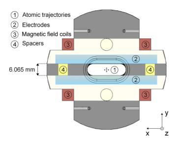
FIG. 6. (Color online) Inbound-atom view of the second collimator plate. This corresponds to a section view of the electrode support of Fig. 4 at the "capacitor" label position. The five dots at the center show the atom trajectory positions considered in the electric-field modeling.
