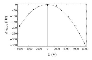
FIG. 11. Quadratic Stark shift of the  $6S_{1/2}$ , F = 3,  $m_F = 0 \rightarrow 6S_{1/2}$ , F = 4,  $m_F = 0$  clock transition frequency determined by the Fourier analysis method. The solid line is a fit with a second-order polynomial.
