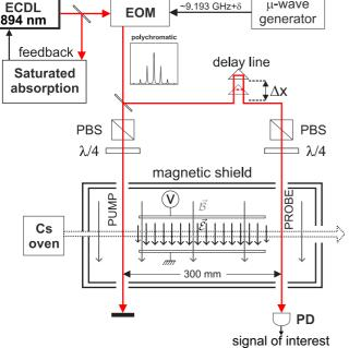
FIG. 3. (Color online) General experimental configuration of the Ramsey interrogation scheme. Details are given in the text.
