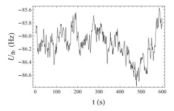
FIG. 13. Typical feedback signal  $U_{\rm fb}$  (calibrated in frequency units) recorded with the microwave frequency locked to the Ramsey fringe center with a voltage of -4.066 kV/cm. The origin of the ordinate is the frequency generated by the microwave generator, corresponding here to 9.192 631 770 GHz.
