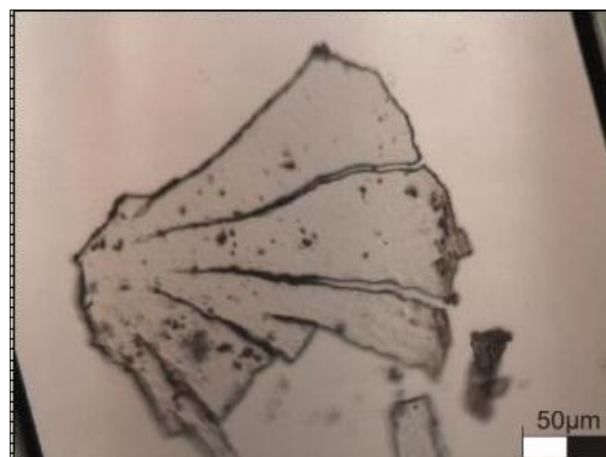
Figure 3-1. Transparent lizardite flake generated by gently pressing loose lizardite powder. Single pieces without cracks were used for the FTIR analysis. The indicated scale corresponds to the \mu\text{m} range.
