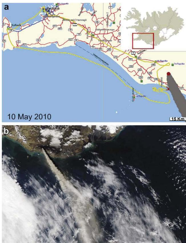
**Fig. 3.** (a) Track of measurement flight on 10 May 2010: Concentration measurements (total suspended particles), dark orange mark on flight track: high ash concentrations (up to  $1800 \mu\text{g m}^{-3}$ ) (b) MODIS Satellite photo of 10 May 2010 (NASA-MODIS, 2010).
