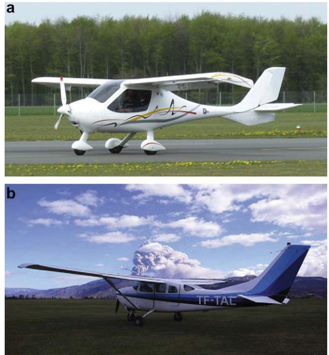
**Fig. 1.** Aircrafts used for the measurements. (a) Flight Design CT: velocity range  $90\text{--}260\text{ km h}^{-1}$ , measurement velocity  $100\text{--}120\text{ km h}^{-1}$ , maximum operation distance 1500 km, typical maximum operation altitude 4500 m. (b) Cessna 206: velocity range  $110\text{--}260\text{ km h}^{-1}$ , measurement velocity  $135\text{--}160\text{ km h}^{-1}$ , maximum operation distance 1500 km, typical maximum operation altitude 5400 m.
