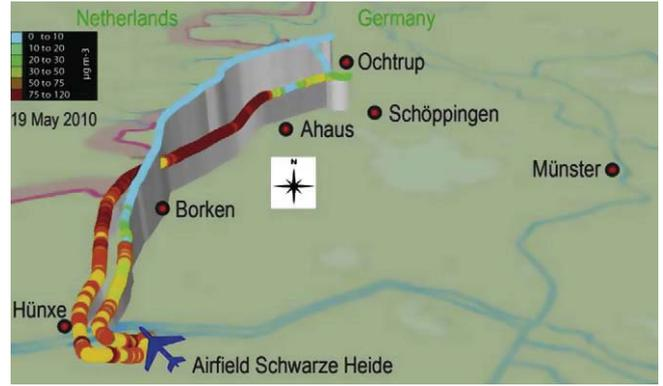
Fig. 16. Track of measurement flight on 19 May 2010 with measured concentration of PM10, colours indicate the concentration range.
