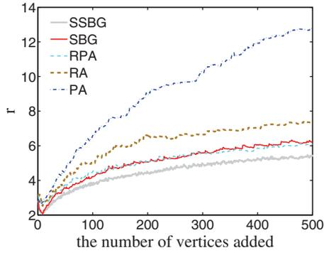
Fig. 4: (Color online) The eigenratio  $\lambda_N/\lambda_2$  as a function of the number of new nodes added. The initial network is an ER random graph with  $N=20$ ,  $\bar{k}=10$ . New nodes are introduced with degree equal to the average degree of the original networks.
