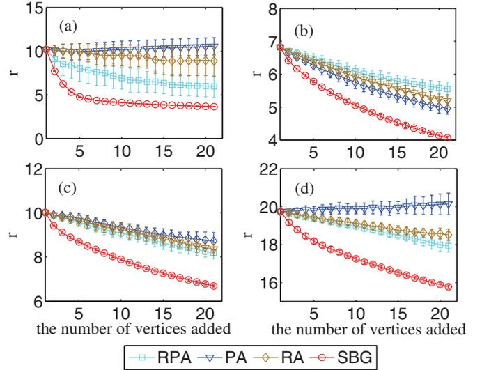
Fig. 1: (Color online) Four growing mechanisms starting from different network models including (a) ER random graph with  $\bar{k} = 15$ , (b) GN benchmark with  $k_{in} = 12$ , (c) WS small-world network with  $p = 0.01$  and  $\bar{k} = 20$ , (d) BA network with  $\bar{k} = 10$ . The initial network size in these four models is 300. The results are obtained by averaging over 20 independent realizations.
