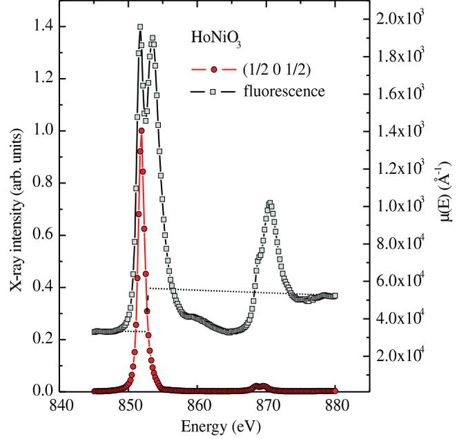
**Figure 2.** Energy dependence of the fluorescence and integrated intensity of the magnetic  $(\frac{1}{2} 0 \frac{1}{2})$  reflection of polycrystalline  $\text{HoNiO}_3$  measured with  $\pi$  incident light at 50 K.
