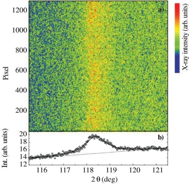
**Figure 1.** (a) Section of the  $(\frac{1}{2} 0 \frac{1}{2})$  resonant magnetic powder diffraction ring of  $\text{HoNiO}_3$  at the Ni  $L_3$  edge (853 eV) and 50 K measured with  $\pi$  incident light. (b) Intensity after vertical integration of the image as a function of  $2\theta$ . The solid line corresponds to a Lorentzian fit with a linear background.
