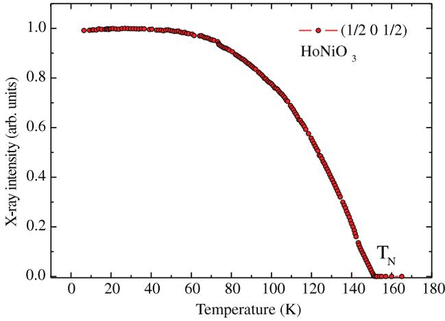
**Figure 3.** Temperature dependence of the integrated x-ray intensity of the magnetic  $(\frac{1}{2} 0 \frac{1}{2})$  reflection taken at the Ni  $L_3$  edge at (852 eV) with  $\pi$ -polarized light incident on polycrystalline  $\text{HoNiO}_3$ . The form of this curve represents the temperature dependence of the Ni magnetic moments only.
