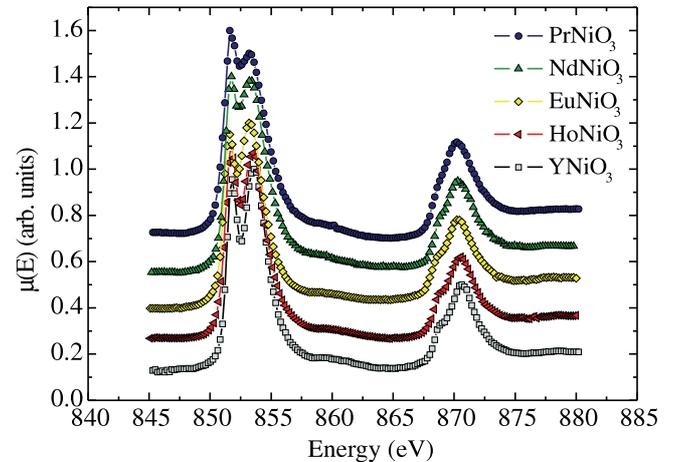
**Figure 7.** Ni  $L_{2,3}$  absorption spectra at about 50 K for  $\text{PrNiO}_3$ ,  $\text{NdNiO}_3$ ,  $\text{EuNiO}_3$ ,  $\text{HoNiO}_3$  and  $\text{YNiO}_3$ . At 50 K all compounds are in the insulating phase.
