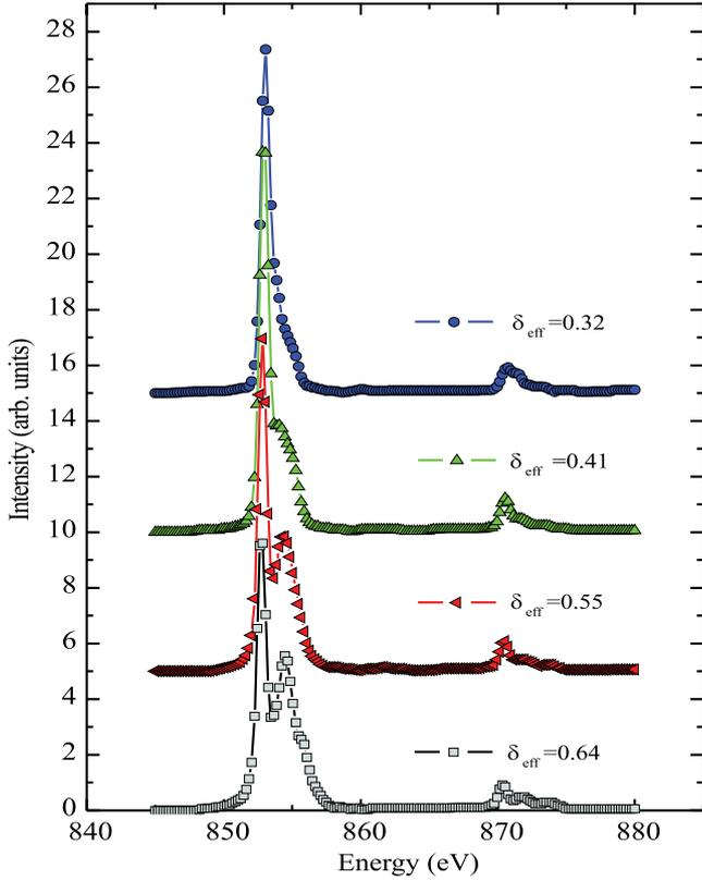
**Figure 5.** Calculated resonant diffraction signal for the magnetic  $(\frac{1}{2} 0 \frac{1}{2})$  reflection of  $\text{RNiO}_3$ . The different spectra are calculated with different charge disproportionation on both Ni-sites.
