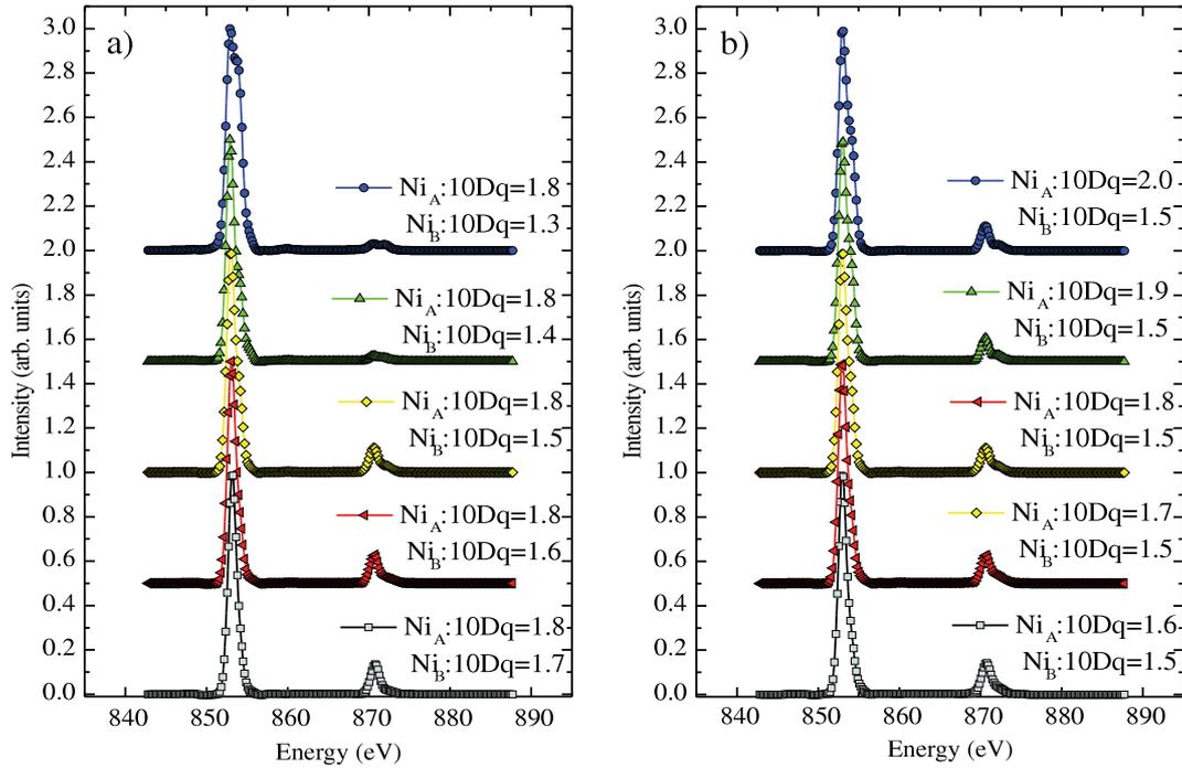
**Figure 6.** Calculated resonant diffraction signal for the magnetic  $(\frac{1}{2} 0 \frac{1}{2})$  reflection of  $\text{RNiO}_3$ . The different spectra are calculated with constant charge disproportionation of  $\delta_{\text{eff}} = 0.32$  and different  $10D_q$  for the  $\text{Ni}_A$ - and  $\text{Ni}_B$ -sites.
