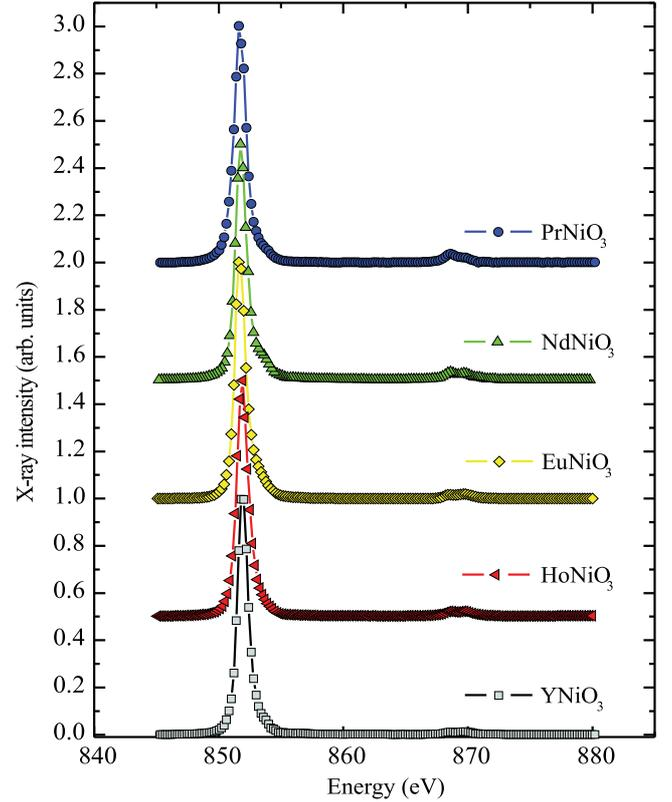
**Figure 4.** Energy dependence of the integrated intensity of the magnetic  $(\frac{1}{2} 0 \frac{1}{2})$  diffraction of polycrystalline samples of  $\text{RNiO}_3$  with R = Pr, Nd, Eu, Ho and Y measured with  $\pi$  incident light at 50 K. The spectra are ordered with regard to increasing ionic radii of the R ion and shifted for easy comparison.
