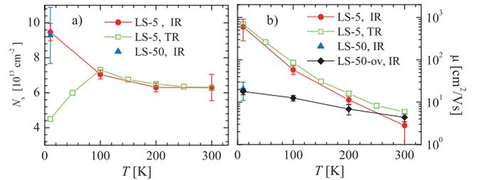
FIG. 2 (color). Comparison of the sheet carrier concentration  $N_s$  (a) and mobility  $\mu$  (b) as deduced from IR (full symbols) and transport (TR, open symbols) measurements. The values deduced from the IR data were calculated using  $m^* = 3.2 m_e$  as discussed in the text. Error bars represent 1 standard deviation.
