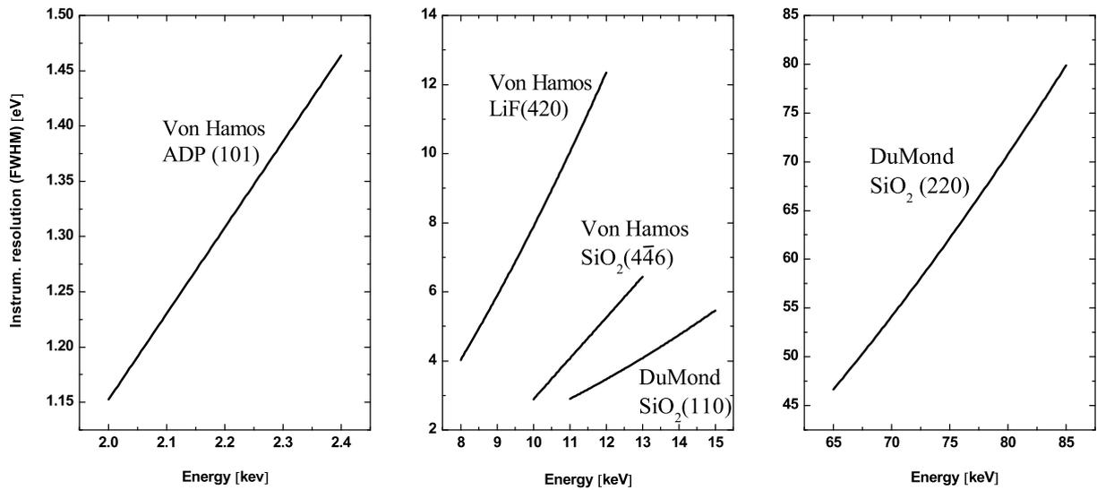
**Fig. 1.** Variation of the FWHM instrumental resolution of the von Hamos and DuMond spectrometers as a function of the X-ray energy. The energy-dependent instrumental broadening is shown for the energy domains corresponding to the measured  $M$  transitions (left panel),  $L$  transitions (mid panel) and  $K$  transitions (right panel).
