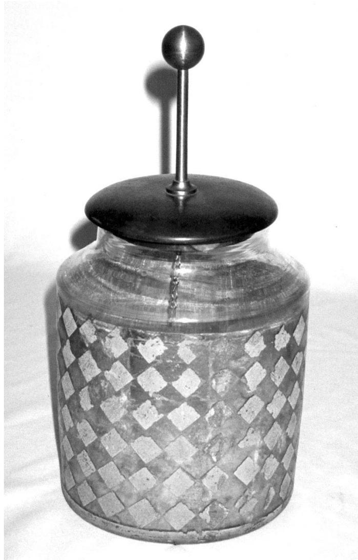
Diamond Jar. The diamond jar adds some drama to the process of charging up a Leiden jar. The tinfoil inner and outer coatings of the jar are made up of diamonds with small spaces between their points. As the jar is charged, sparks jump between the points of the diamonds. The device is also called a Spangled Jar. This example is at Case Western Reserve University. (Photograph and Notes by Thomas B. Greenslade, Jr., Kenyon College)
