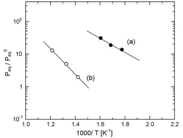
Fig. 7. Van't Hoff plots for (a) Li[BH<sub>4</sub>] with MgCl<sub>2</sub> after heat treatment at 593 K and (b) pure Li[BH<sub>4</sub>]. Equilibrium pressures of (a) and (b) are obtained from PC desorption isotherms in Fig. 5, from ref. [17], respectively.
