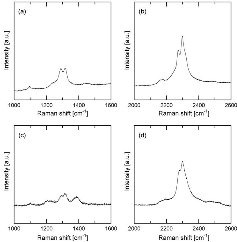
Fig. 3. Raman spectra of pure Li[BH<sub>4</sub>] (a and b) and Li[BH<sub>4</sub>] with MgCl<sub>2</sub> after heat treatment at 593 K under 10 MPa of hydrogen (c and d).
