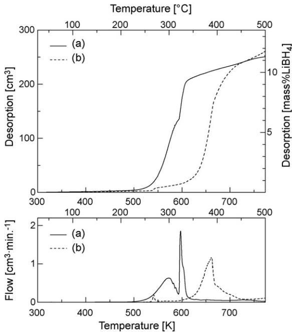
Fig. 4. Temperature programmed desorption spectra of: (a) Li[BH<sub>4</sub>] and MgCl<sub>2</sub> mixture after heat treatment at 593 K under 10 MPa of hydrogen; (b) pure Li[BH<sub>4</sub>]. The samples were heated after evacuation at room temperature with a heating rate of 0.2 K min<sup>-1</sup>. The upper graph and the lower graph show the desorbed gas volume and the gas flow as a function of temperature, respectively.
