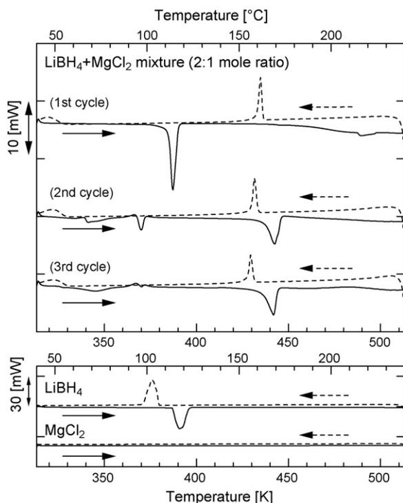
Fig. 1. Differential scanning calorimetry profiles of  $\text{Li}[\text{BH}_4]$  and  $\text{MgCl}_2$  mixture with a sealed sample cell. The heating rate is  $5 \text{ K min}^{-1}$ . Measurements with pure  $\text{Li}[\text{BH}_4]$  and  $\text{MgCl}_2$  were also performed at the same heating condition. Solid lines and dotted lines show heating and cooling, respectively. A total of 5 mg of the sample was used for each measurement.
