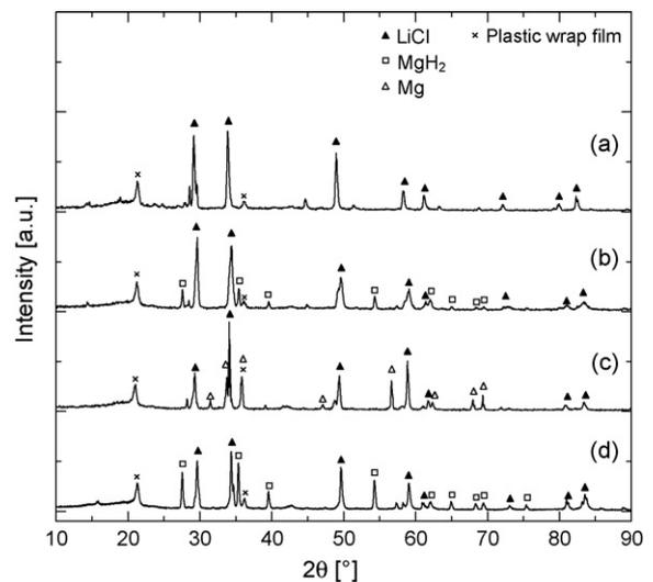
Fig. 8. Powder X-ray diffraction profiles of Li[BH<sub>4</sub>] and MgCl<sub>2</sub> mixture: (a) after heat treatment at 593 K for 3 h, (b) after desorption in vacuum to 593 K, (c) after desorption in vacuum to 623 K and (d) after absorption up to 10 MPa of hydrogen at 623 K, respectively.
