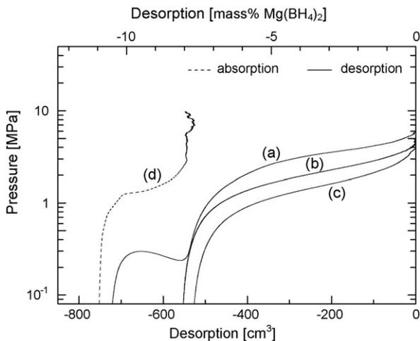
Fig. 6. Absorption/desorption isotherms for Li[BH<sub>4</sub>] and MgCl<sub>2</sub> mixture after heat treatment at 593 K: (a) desorption at 563 K; (b) desorption at 593 K; (c) desorption at 623 K; (d) absorption at 623 K. Curve (d) was measured after the desorption measurement at the same temperature.
