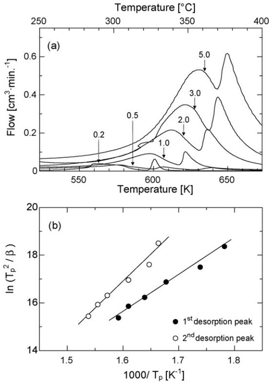
Fig. 5. (a) Temperature programmed desorption spectra of Li[BH<sub>4</sub>] and MgCl<sub>2</sub> mixture after heat treatment at 593 K under 10 MPa of hydrogen. Numbers shown in the graph indicate the heating rate in K min<sup>-1</sup>. A total of 20 mg of the sample was used for the measurements. (b) Kissinger plot of thermal desorption spectra at a heating rate of 0.2–5.0 K min<sup>-1</sup>, where T<sub>p</sub> is a peak temperature of the spectra and β is a heating rate.
