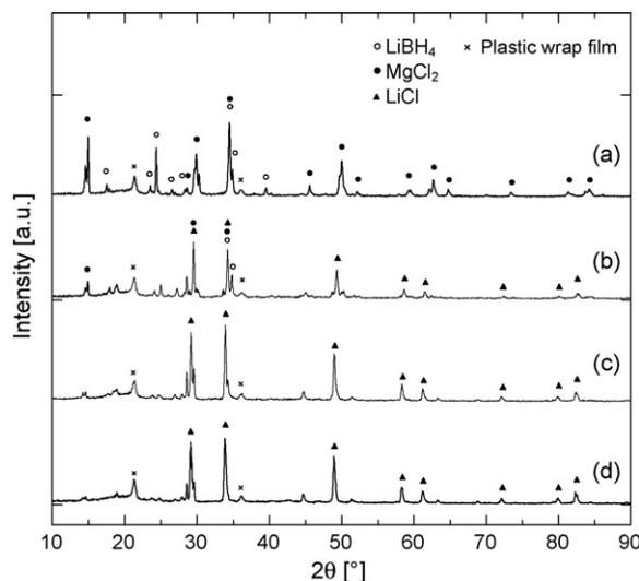
Fig. 2. Powder X-ray diffraction profiles of  $\text{Li}[\text{BH}_4]$  and  $\text{MgCl}_2$  mixture: (a) before heat treatment; (b) after heat treatment at 453 K; (c) after heat treatment at 523 K; (d) after heat treatment at 593 K, respectively. Each heat treatment was carried out under 10 MPa of hydrogen.
