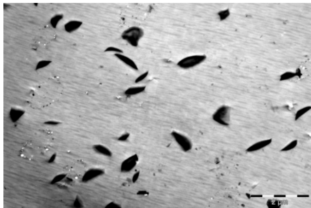
Figure 3. OsO 4 -stained TEM micrograph showing the structure of a blend formed by 90 wt % polystyrene homopolymer and 10 wt % PPV. The elongated shape of the dark PPV domains suggests that nucleation and growth occurs via subsequent stacking of PPV rods, rather than following an isotropic radial growth.
