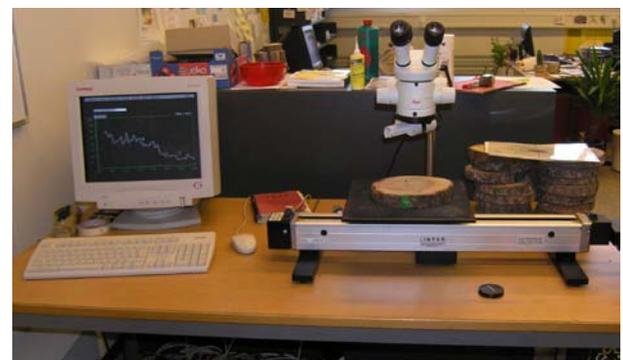
**Fig. A3.12** LINTAB positioning table coupled to a Leica stereomicroscope and TSAP software was used for the measurement of tree-ring width.
