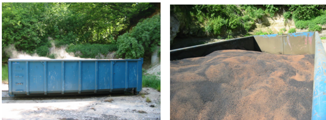
Figure 10.3: At the end of the first storage experiment (Blank 1), the smouldering granules were poured in a 25\text{ m}^3 open bucket, from which smokes were still emitted (left). The material kept on burning during several weeks and iron oxidized to red iron oxide (right)
