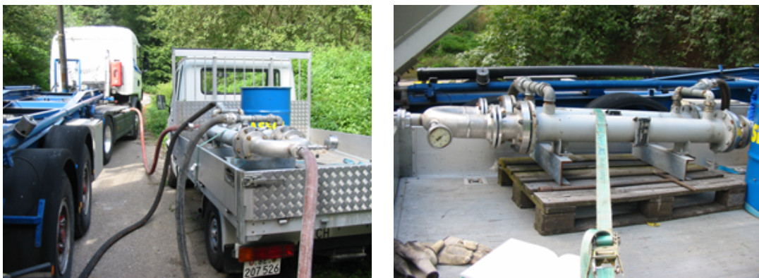
Figure 11.1: Compressed air provided by the truck was connected to a heat exchanger in order to obtain cooled compressed air
