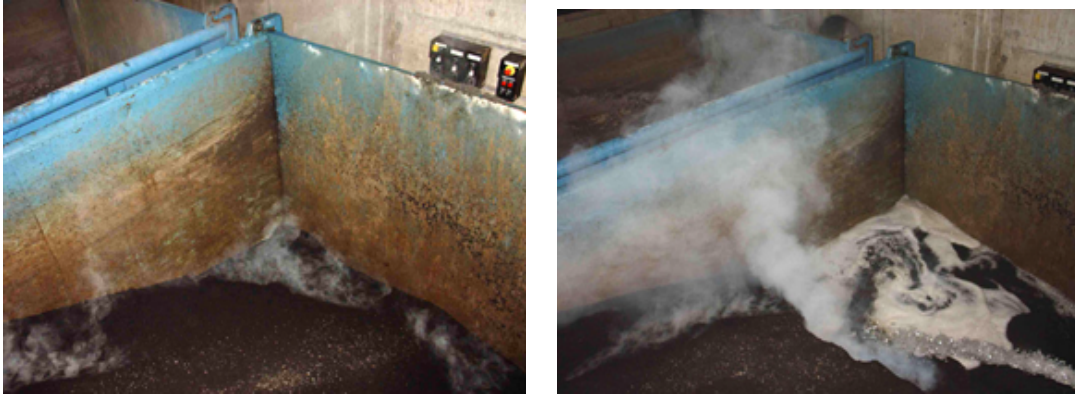
Figure 10.5: Smouldering fire of a remaining batch of dried granules treated with a sodium hypophosphite solution as antioxidant processing. The fire occurred one week after having been placed in a 25 m 3 open bucket (left) and was extinguished by water addition (right)
