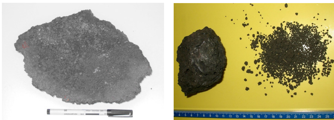
Figure 7.1: Smouldering fire causes the formation of large piece of agglomerated granules (left) and smelt residue from sewage granules (right)
