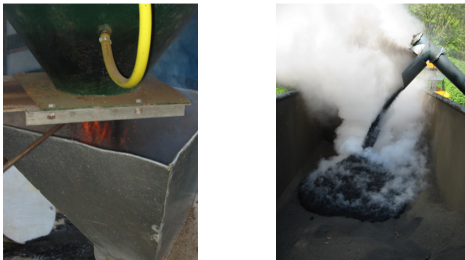
Figure 10.8: The smouldering granules caught fire due to the fresh air contact during the emptying of the silo (left) and the draining of the very hot granules into the bucket (right)
