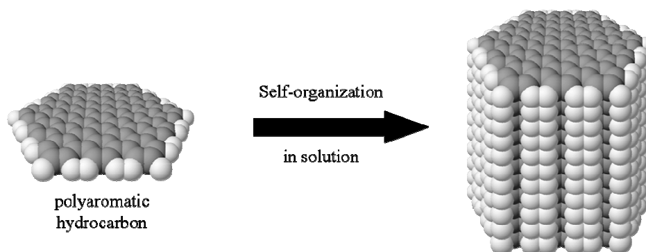
Figure 5.1 – Sketch of a molecular wire formed by self-assembling of individual PAHs
