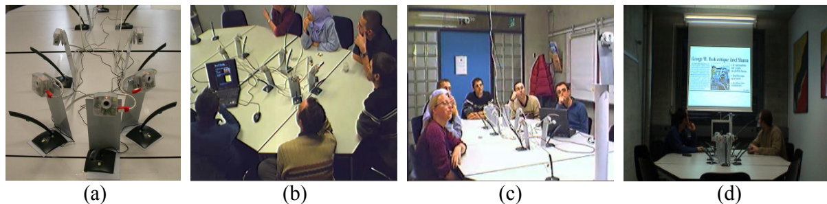
Fig. 3.2. Snapshots of the document-centric Smart Meeting Room : (a) FireWire web-cam and Labtec microphone pair per participant, (b) overview from a web-cam capturing meeting, (c) another overview web-cam positioned diagonally opposite and (d) a web-cam focused on the projector's screen.
