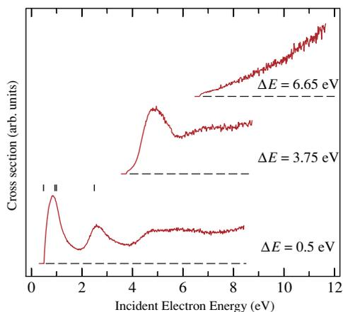
**Figure 3.** Excitation functions of phenyl azide. Bottom: pure vibrational excitation, centre: excitation of a triplet state, top: excitation of a dipole-allowed singlet–singlet transition. Vertical bars indicate the attachment energies estimated from the virtual orbital energies using the empirical scaling relation of Chen and Gallup [27].
