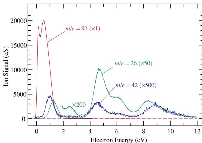
**Figure 4.** Dissociative electron attachment spectra of phenyl azide.
