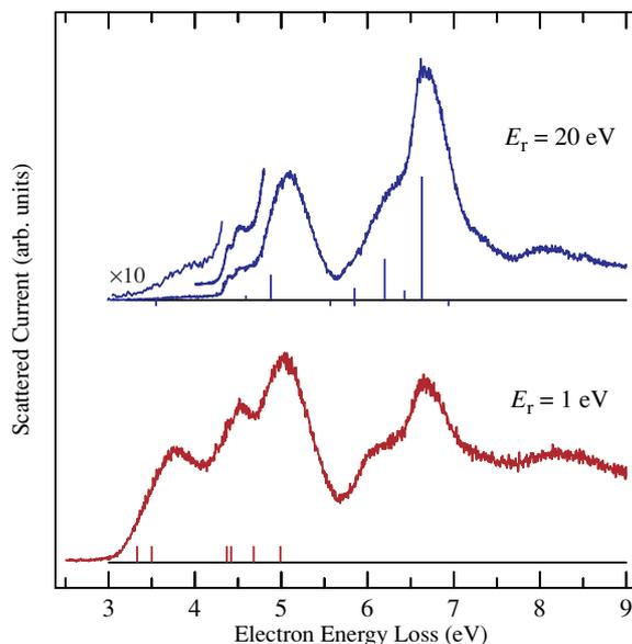
**Figure 2.** Electron energy-loss spectra of phenyl azide. Top: conditions emphasizing singlet–singlet transitions, bottom: conditions emphasizing singlet–triplet transitions. Bars below the top spectrum indicate calculated transition energies and dipole intensities (transitions with an oscillator strength of less than  $f = 0.02$  are indicated by a tick below the baseline for clarity). Bars below the bottom spectrum indicate calculated singlet–triplet transition energies.
