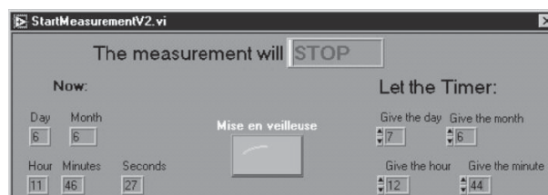
Figure 11: GUI of the developed program in order to control the timer of the QCM. In this case the stop of the measurement is defined.
