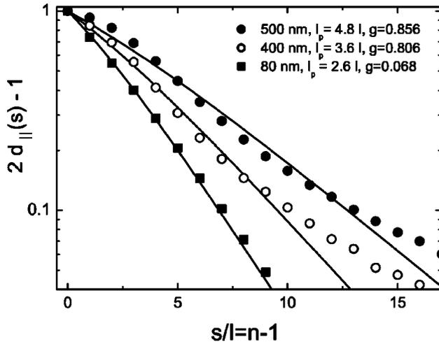
Fig. 2. Depolarization of multiply scattered light:  $2d_{||}(s) - 1$  from theory [Eq. (4), curves] and simulation (symbols). Excellent agreement is found for Rayleigh scatterers, while for larger particles the agreement becomes somewhat less good.
