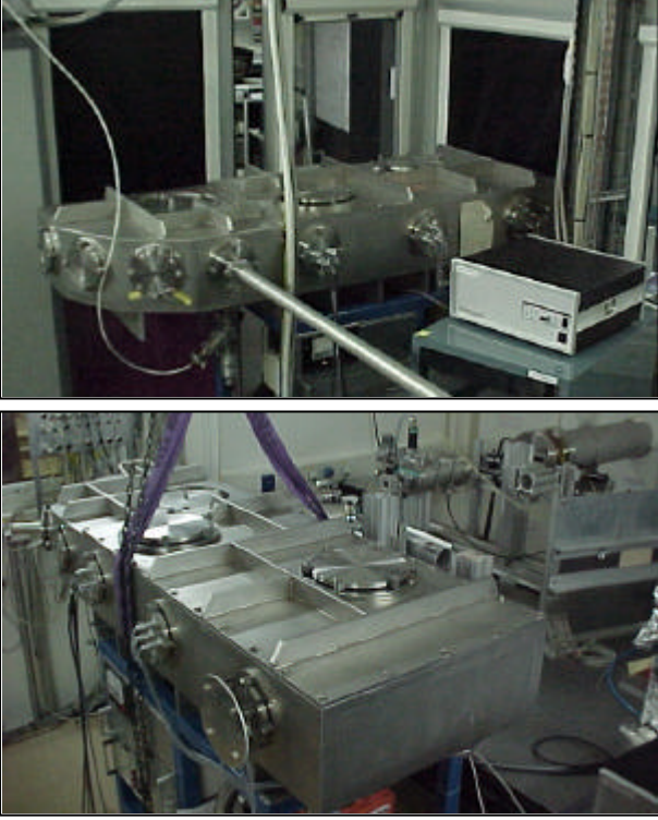
FIG. 2: Photographs of the von Hamos spectrometer as installed at the ESRF beamline ID21 (top) and BM5 (bottom). Due to the higher x-ray beam energies employed at BM5, no evacuated pipe was needed to connect the spectrometer chamber to the exit window of the beam-line (pipe emerging from the wall on the right). One sees that at BM5 the spectrometer chamber was rotated by 180 deg. around a vertical axis with respect to the set-up employed at ID21.
