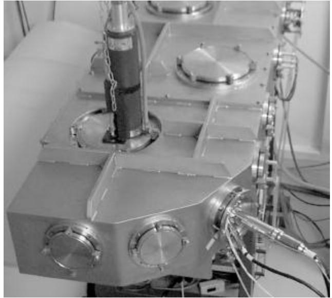
Fig 1. Photograph of the Von Hamos spectrometer. The three circular ports on the top part of the spectrometer chamber permit access to the target, crystal, and CCD detector. The vertical device on the target port is the 100 kV x-ray tube. Also visible at the bottom of the photograph, on the right, is the 20 kV electron gun mounted horizontally on one of the four beam ports.
